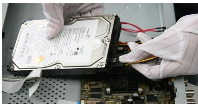
4. Place the HDD on the bottom of the device and then fasten the screws on the bottom to fix the HDD.
